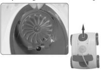
5.1 To adjust the direction of the robot, rotate the outlet cover. The direction of the robot will be determined by the position of the indicator.
