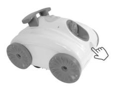
6.1 Press in the button at the front of the cleaner and lift up the top shell. Continue to lift up the shell until you hear a "click" at the hinge and the shell stays in place.
