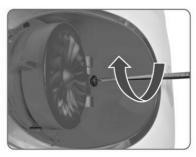
5.2 To adjust the speed of the robot, use a screw driver to turn the screw at the bottom of the cover. Screwing out increases the speed and screwing in decreases the speed.
