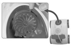
Note: with indicator on vertical position, the robot will go straight ahead. With indicator turned right, the robot will go left. With indicator turned left, the cleaner will go right.
