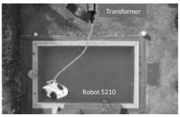
4.1 Place your power box to a midpoint between the two ends of your pool and at least 3.50 m from the edge of the pool.
