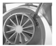
7.2: Use a flat screw driver to ply the flap assembly out as shown
